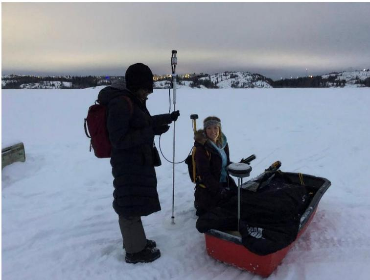
Fig.1: Collecting snow depth and ice thickness using magnaprobe and ground penetrating radar (GPR) on Vee Lake, Northwest territories, November 29, 2021.
